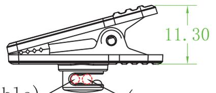
(inner section for  $\phi 2.0$  cable) (outer section for  $\phi 2.5$  cable)
